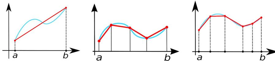
Figure 12: Trapezoidal approximation with increasing discretization
