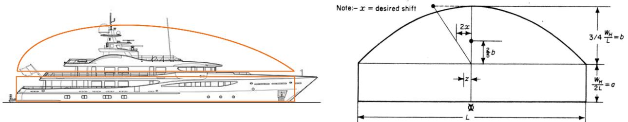
Figure 5: Illustration and formula representation of the parabolic approximate loading method [5]
