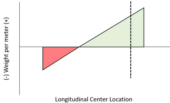
Figure 8: Negative trapezoidal loading representation due to extreme LCG placement
