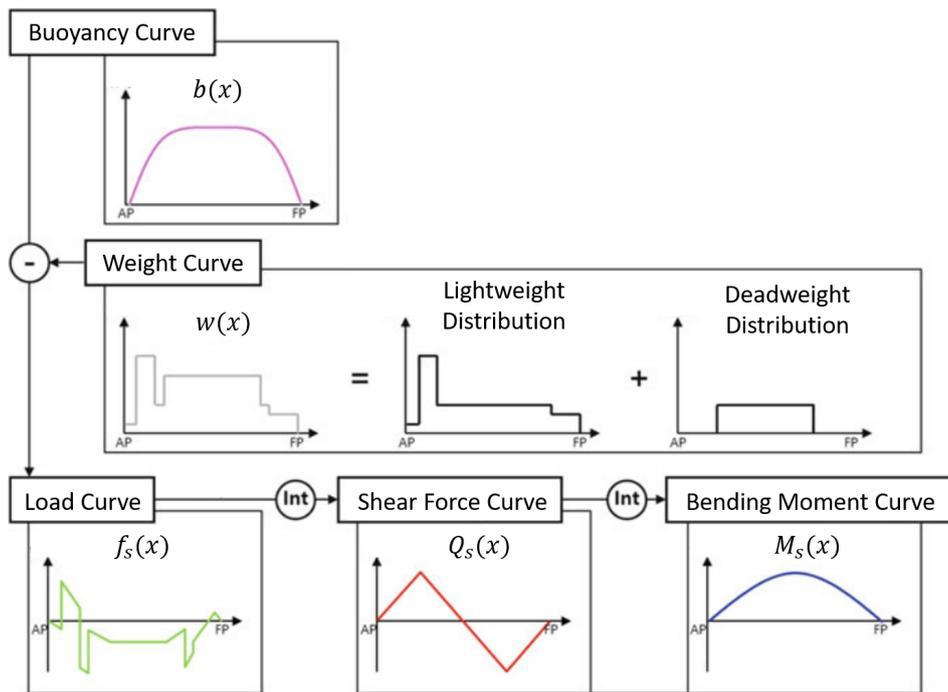
Figure 4: Still water bending moment general calculation process [9]
