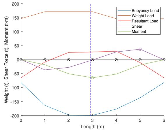
Figure 16: Aligned LCB & LCG
