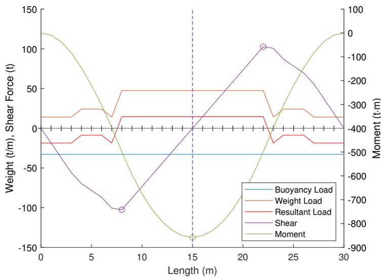
Figure 22: Trapezoidal distributed shear and bending moment results (n=5)
