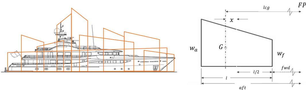
Figure 7: Illustration and trapezoidal representation of the direct loading method
