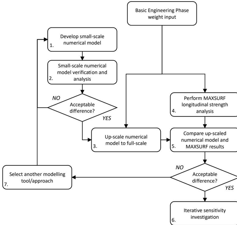
Figure 11: General framework and process flow chart for longitudinal strength assessment
