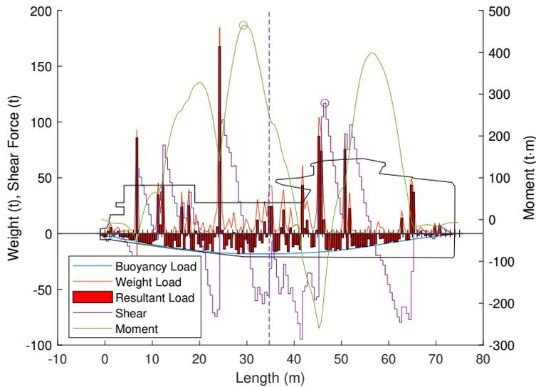
Figure 31: Single-point grouping shear and bending moment results (n=2)
