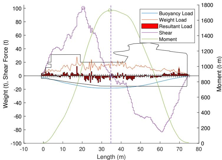
Figure 32: Multi-point grouping shear and bending moment results (n=2)
