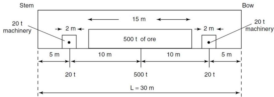
Figure 17: General barge schematic with loading and locations [3]
