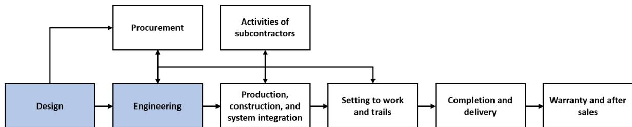
Figure 2: Standard main process for a ship’s new building program [17]
