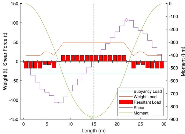
Figure 21: Multi-point grouping shear and bending moment results (n=1)
