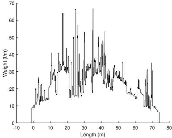
Figure 26: MAXSURF weight distribution
