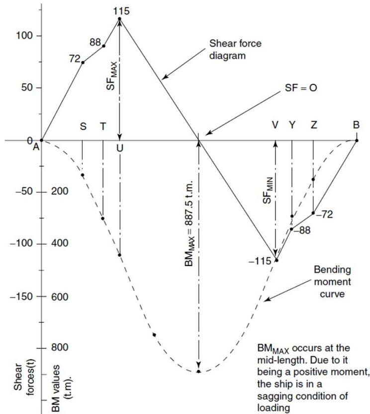
Figure 18: Shear force and bending moment analytical results [3]
