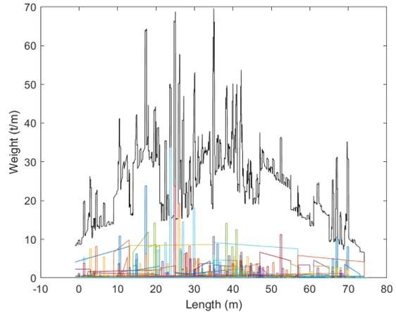
Figure 27: MATLAB trapezoidal weight distribution
