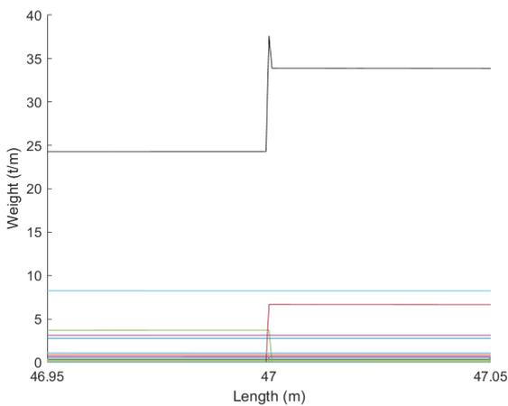
Figure 28: Trapezoidal discretization error
