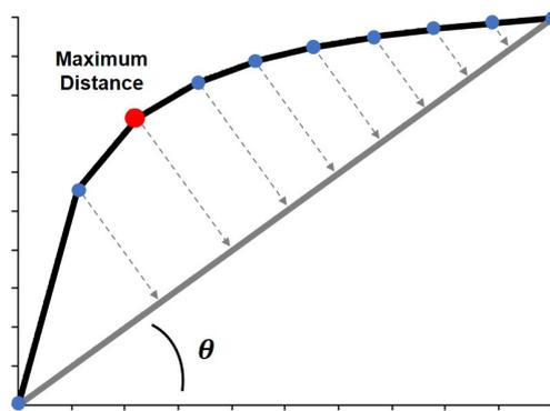
Figure 38: Triangle threshold general process [10]
