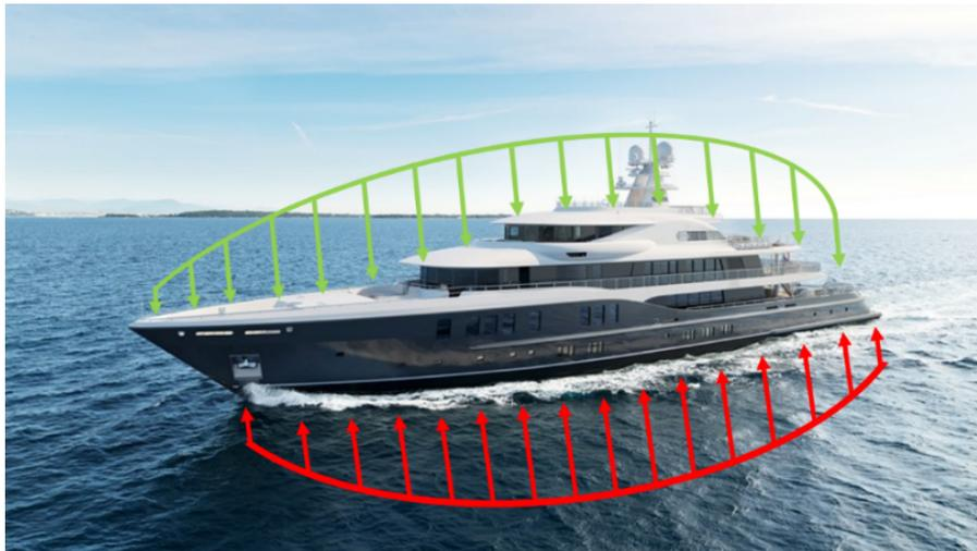
Figure 1: Loading and buoyancy distribution in the 74.00m AMELS 242
