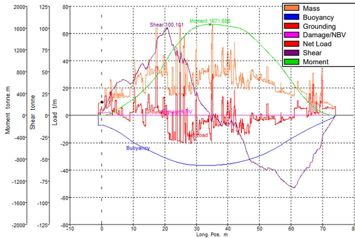
Figure 24: MAXSURF shear and bending moment output results
