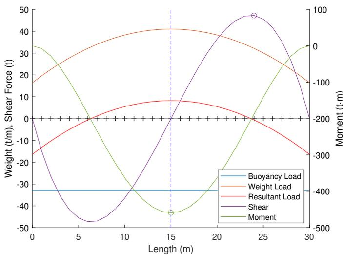
Figure 19: Parabolic distributed shear and bending moment results (n=10)
